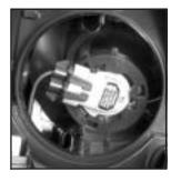
Disconnect the wiring harness, then turn the bulb socket counterclockwise to remove it.
